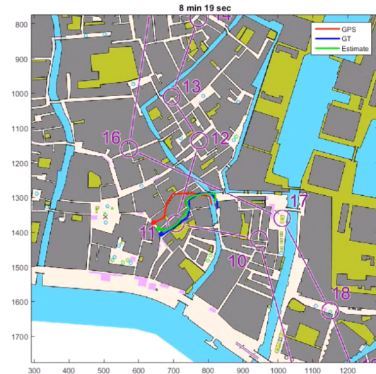
Fig. 1. A snapshot from the world championship in sprint orienteering in Venice 2014. Soren Bobach is on his way to victory, and the live public can watch the red trajectory based on map matching of GPS data sampled with several seconds sampling time. The blue line shows his own reconstruction (can be seen as ground truth), while the green one is based on a particle filter supported by map information, see [1].
